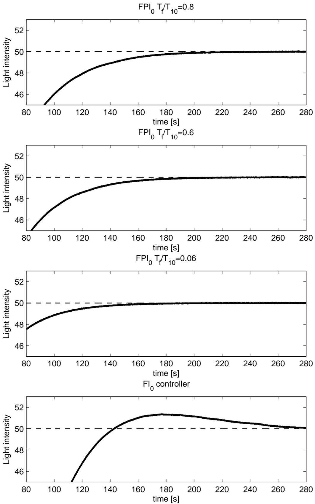
Figure 3.41: Experimental results detail – delayed system output, setpoint step
