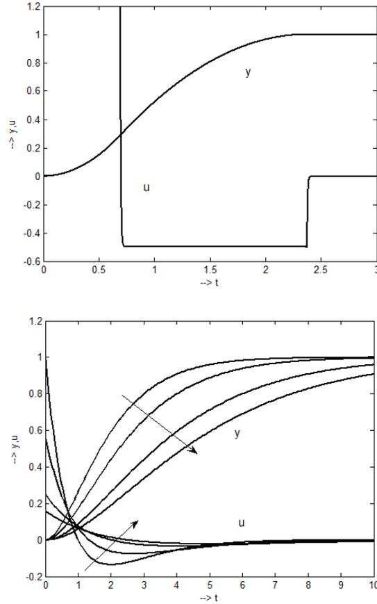
Figure 1.18: Output and control signal transients of double integrator plant: left - for the relay MTC with control signal constrained by  $U_{max} = 1.2$  and  $U_{min} = -0.5$ ; right - for linear pole assignment control with double real pole values  $-1, -0.75, -0.5$  and  $-0.4$  arrows indicate pole shifting to zero (i.e. slowing down transients)
