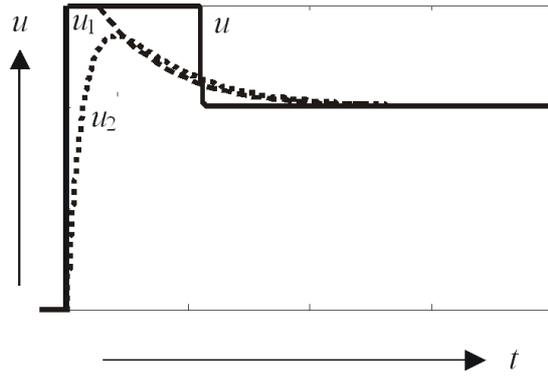
Figure 1.16: DC1: Control signal reaction to a setpoint step change;  $u$  – time optimal (without rate constraints),  $u_1$  – with rate constraints for the transient from the limit to the steady state value,  $u_2$  – as  $u_1$ , with an additional limit on the control signal increase.
