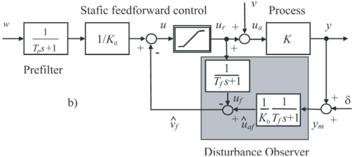
Figure 3.17: FI<sub>0</sub>-controller, structure equivalent for  $T_p = T_f$  to I-controller
