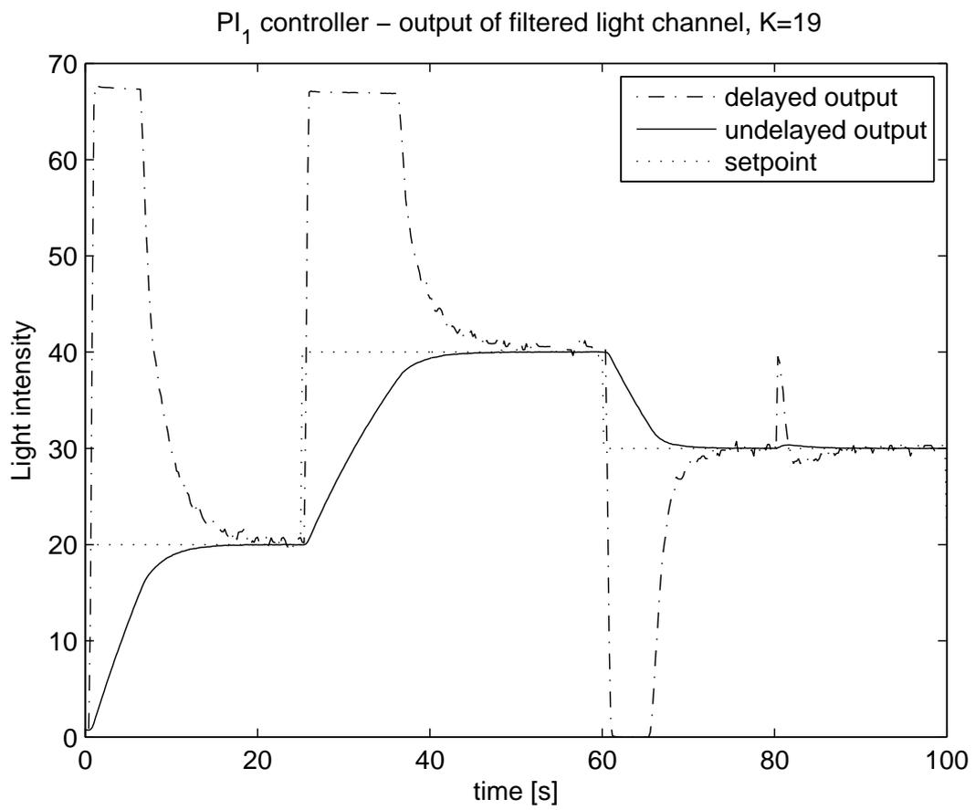
Figure 3.47: PI<sub>1</sub>-controller, filtered light channel control for  $K = 19$
