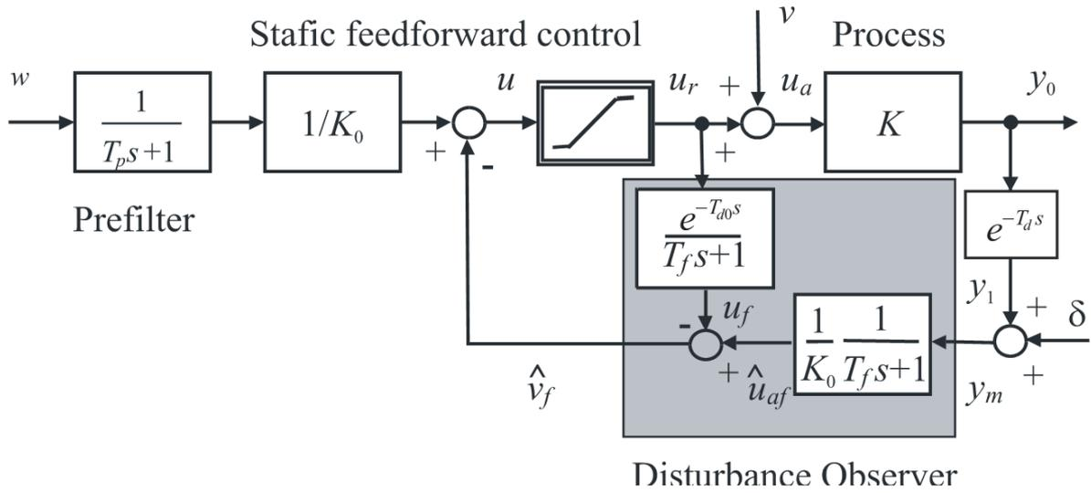
Figure 3.27: FPrI<sub>0</sub>-controller
