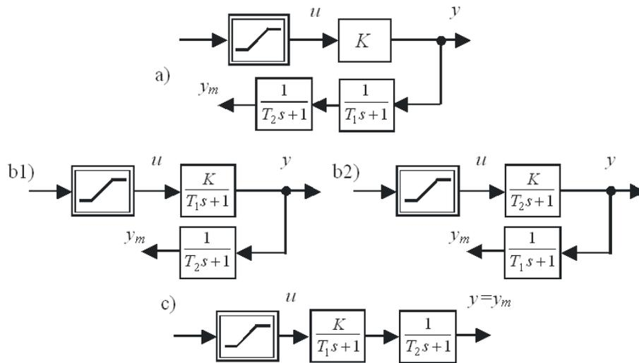
Figure 1.21: Control loops with the 2<sup>nd</sup> order dominant dynamics and the relative degrees: a) 0; b) 1 and c) 2.
