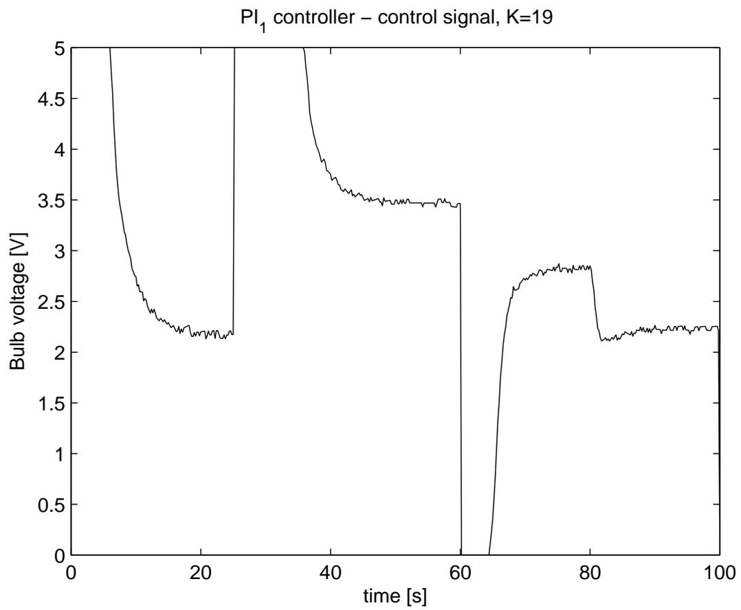
Figure 3.48: PI<sub>1</sub>-controller, filtered light channel control for  $K = 19$
