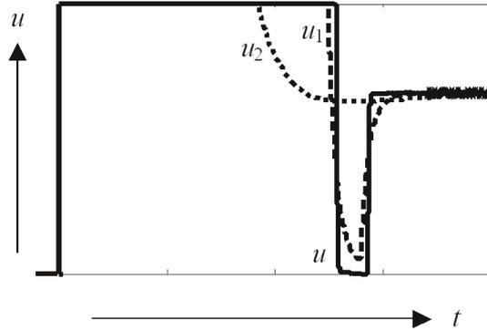
Figure 1.17: DC2: Control signal reaction to a setpoint step change;  $u$  – time optimal (without rate constraints),  $u_1$  – by limiting rate of changes in transient from one control limit to the opposite one and in transient to the steady state,  $u_2$  – as  $u_1$  but with stronger constraints.
