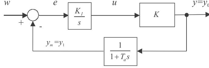
Figure 2.5: Loop with I controller, memoryless plant and non-modelled dynamics approximated by time constant
