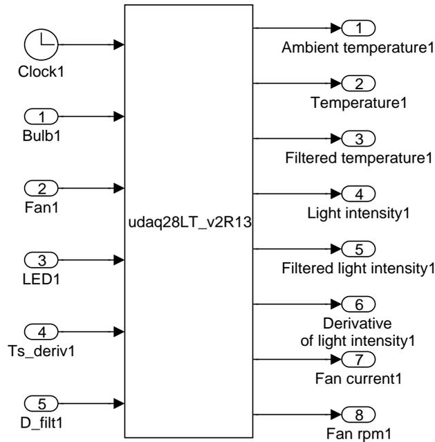
Figure 3.7: Communication interface block in Simulink
