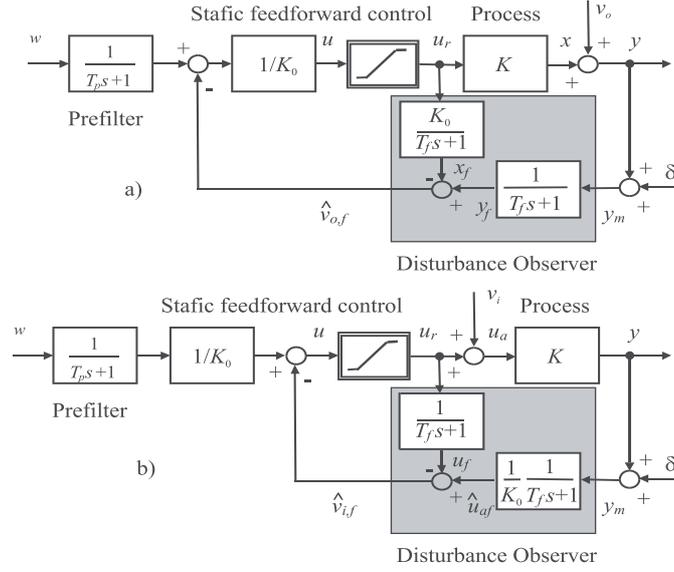
Figure 2.1: FI<sub>0</sub> controllers: static feedforward control extended 1) by reconstruction and compensation of (a) output and (b) input disturbances of a memoryless plant and 2) by a prefilter; in nominal case  $K_0 = K$
