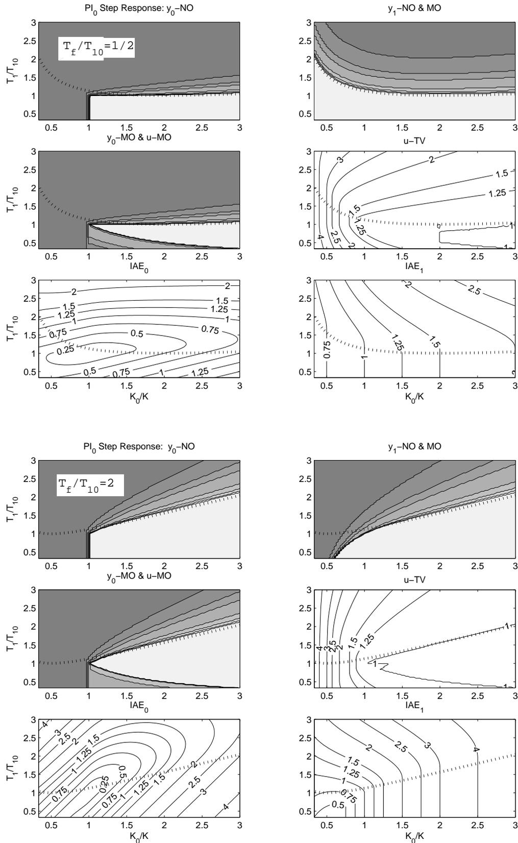
Figure 2.14: Performance portrait of the  $PI_0$ -IM controller for setpoint response with two values of  $\tau_f = 1/2$  and  $\tau_f = 2$  and different measurement precisions  $\epsilon_y = \{0.1, 0.05, 0.02, 0.01, 0.001, 0.0001, 0.00001\}$  with white showing the best performance; dotted border of complex poles (2.50), (2.52)
