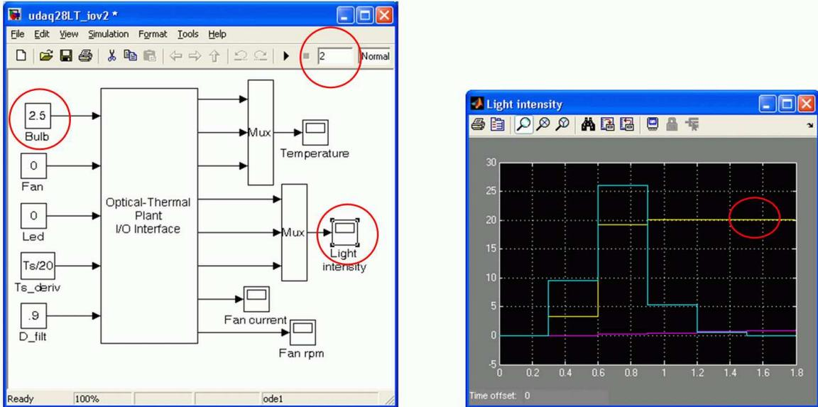
Figure 3.10: Basic Simulink model for the udaq28/LT plant
