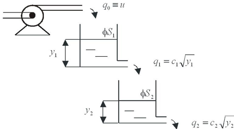
Figure 1.22: Two tank system with a “noninertial” pump
