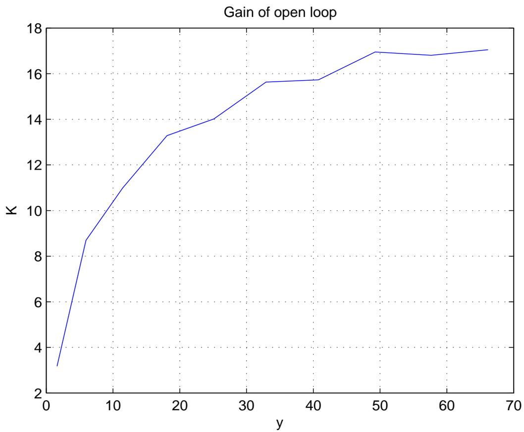
Figure 3.14: Process gain in multiple operating points as function of the output variable
