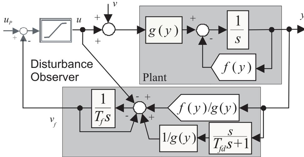
Figure 5.2: Rejection of the input disturbances  $v$  by correction of the P controller output in the nonlinear  $PI_1$  controller for system  $dy/dt = g(y)(u + v) - f(y)$
