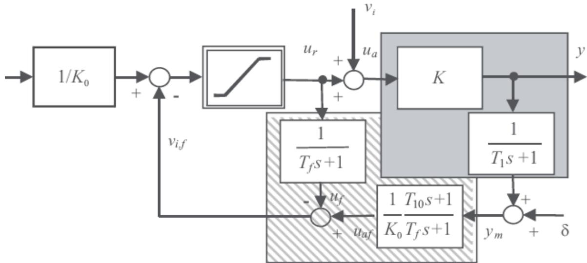
Figure 3.33: FPI<sub>0</sub> controller
