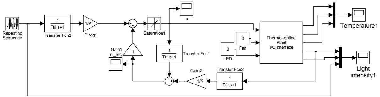
Figure 3.18: FI<sub>0</sub>-controller – Simulink model
