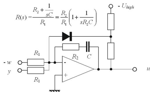
Figure 1.2: Analog electronic PI controller
