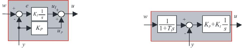
Figure 1.5: I-P controller (left) and the equivalent PI controller with prefilter (right),  $K_I = K_P/T_I$
