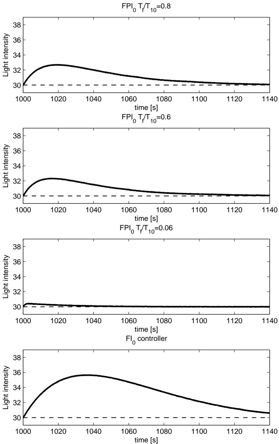
Figure 3.43: Experimental results detail – delayed system output, disturbance step
