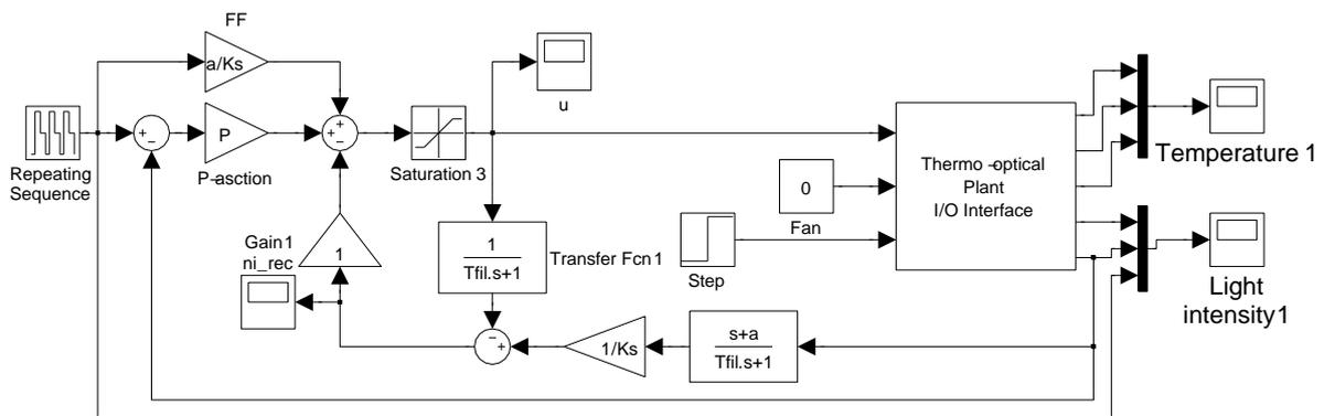
Figure 3.46:  $PI_1$ -controller, Simulink model
