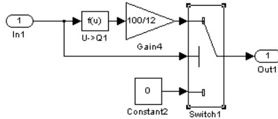
Figure 4.7: Pump implementation in simulink.
