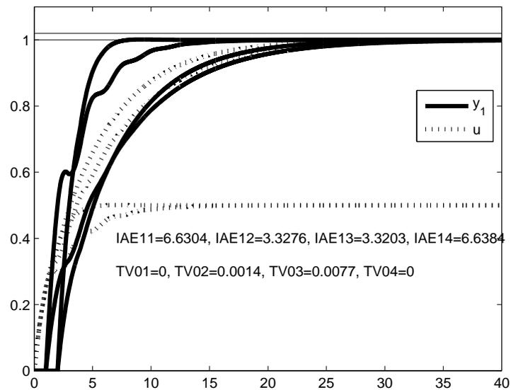
Figure 2.22: Result for seeking an optimal UB of the plant (2.68) with  $K_{min} = 1, K_{max} = 2, T_{d,min} = 1, T_{d,max} = 2$  over PP of 61x61x11 points, areas of  $\epsilon_y$ -MO output step responses identified for tolerances  $\epsilon_y = \{0.1, 0.05, 0.02, 0.01, 0.001, 0.0001, 0.00001\}$ , white denoting the best performance, with identified parameters  $T_f = 1.3796, K_0 = 2.005$  and  $T_{d,0} = 1.8519$  (above) and the corresponding transients (below)
