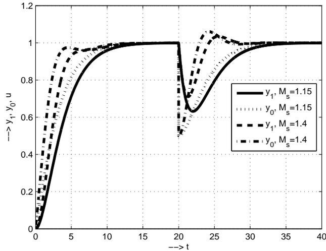
Figure 2.8: Loop with the  $FI_0$  controller and plant (2.22) with  $T_p = T_f$  and  $T_f$  corresponding to (2.27) that yields  $M_s = 1.15$  and with the tuning (2.30) corresponding to  $M_s = 1.4$
