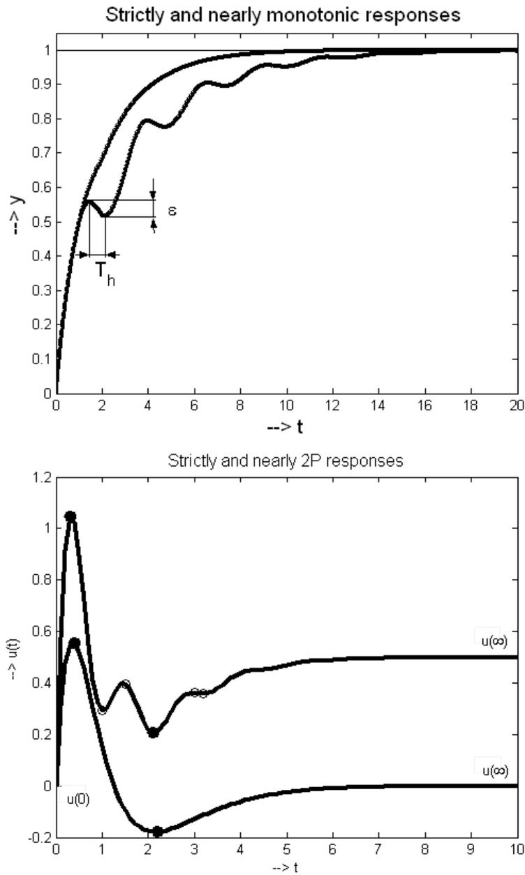
Figure 1.13: Above: Strictly monotonic signal satisfying (1.12) and “nearly monotonic” signal satisfying (1.18) with  $K = T_h/T$ ,  $T$  being the sampling period, is chosen to cover at least one quarter-period  $T_h$  of possible high-frequency signal superimposed on the dominant monotonic signal  $\varepsilon = \varepsilon_y$ ; Below: Nearly and strictly 2P responses; local extreme points denoted by “o” and significant extreme points denoted by “●”
