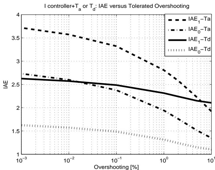
Figure 2.6: IAE1 and IAE0 values versus tolerated overshooting for the time constant  $T_a$  and dead time  $T_d$  according to Tab. 2.1 and Tab. 2.2
