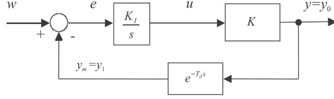
Figure 2.3: Loop with I controller, memoryless plant and dead time
