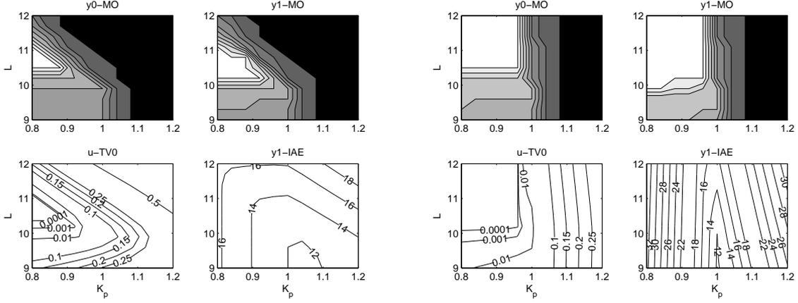
Figure 2.10: PP of the plant (2.38) with the FSP controller based on (2.39)-(2.40) with  $T_f = L_n/2$  (left) and  $T_f = 10L_n$  (right);  $\epsilon_y$ -MO areas identified for tollerances  $\epsilon_y = \{0.1, 0.05, 0.02, 0.01, 0.001, 0.0001, 0.00001\}$  with white denoting the best performance
