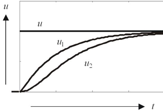
Figure 1.15: DC0: Control signal reaction to a setpoint step;  $u$  – without rate constraints,  $u_1$  – with a rate constraint,  $u_2$  – with constrained 2<sup>nd</sup> derivative of the control signal
