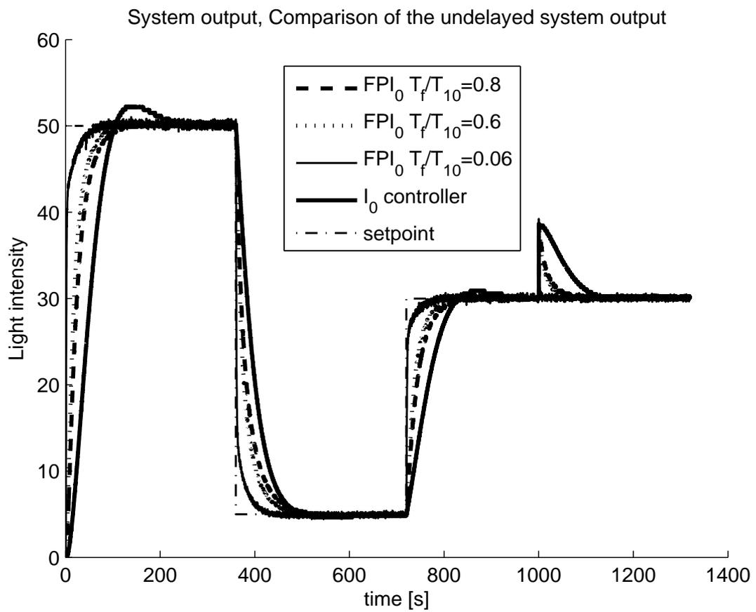
Figure 3.39: Experimental results – undelayed system output
