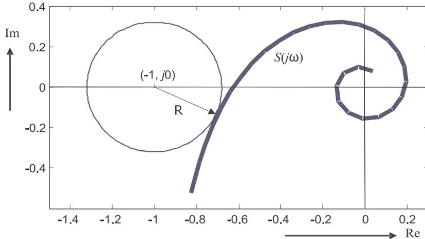
Figure 2.7: Maximal sensitivity  $M_s = 1/R$  is defined as reciprocal value of the maximal radius  $R$  of the circle with centre in critical point  $(-1, 0j)$  that is touging Nyquist curve  $L(j\omega)$
