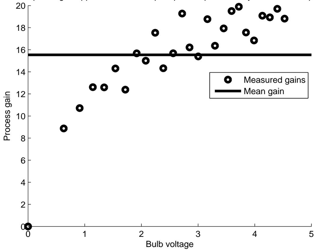
Figure 3.35: Process gain in several operation points as function of the plant input
