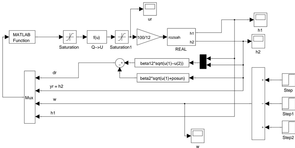
Figure 5.7: Control structure for nonlinear PD1 implemented in Matlab / Simulink. Matlab function block call PD2(u(1), u(2), u(3), u(4))
