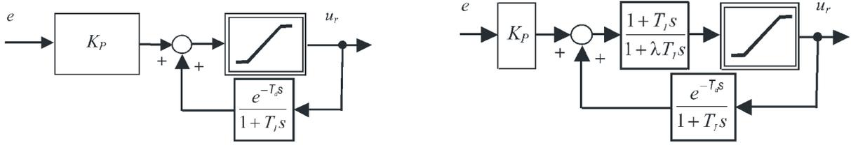
Figure 1.6: Predictive PI controller (PPI) (left) and extended by the IMC controller (right)
