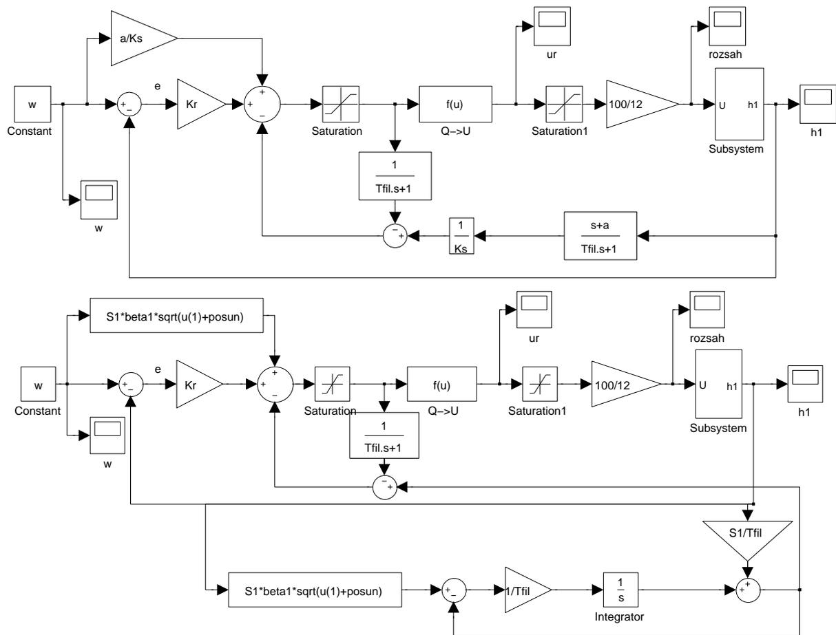
Figure 5.4: Control structure for linear and nonlinear PI1 implemented in Matlab / Simulink
