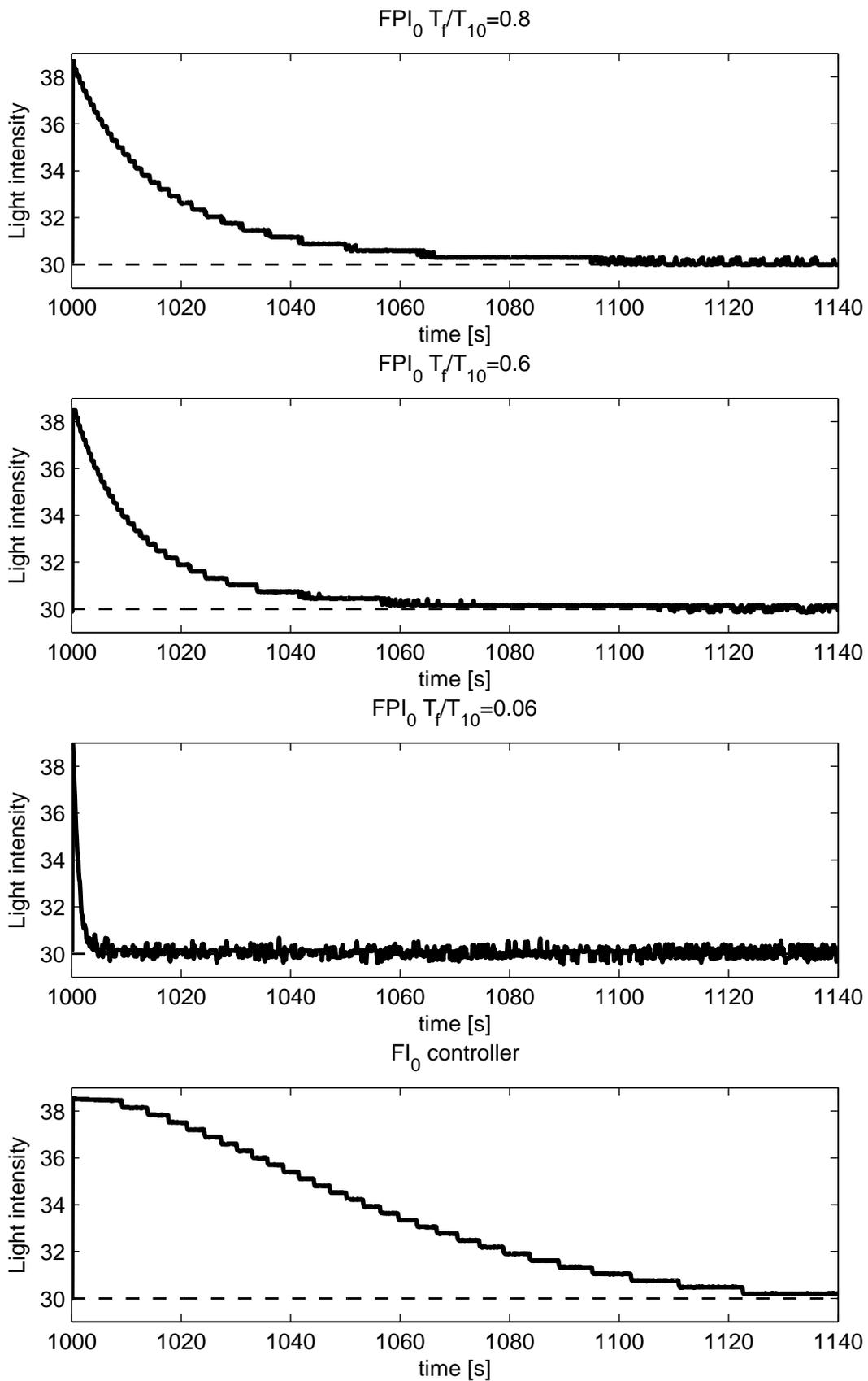
Figure 3.44: Experimental results detail – undelayed system output, disturbance step
