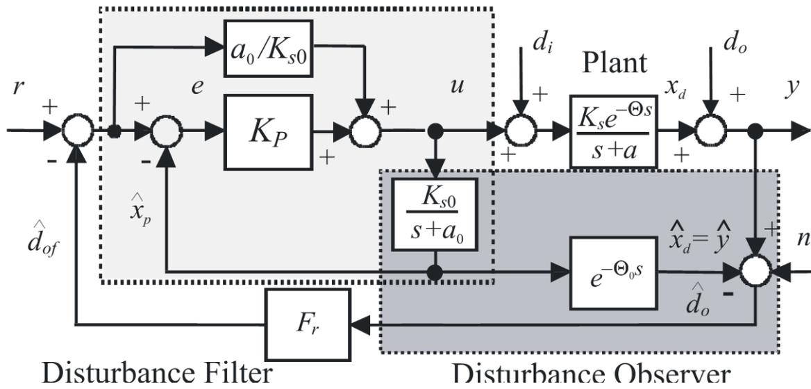
Figure 3.51: Modified P-FSP with the primary loop using 2DOF P-controller with the disturbance filters
