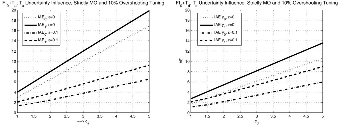
Figure 2.9:  $T_a$  uncertainty influence on average IAE values of outputs  $y_0$  and  $y_1$  for strictly MO tuning ( $K_I = 0.25/(KT_{a,max})$ ) and tuning with 10% tolerable overshooting of  $y_0$  with  $K_I = 0.57/(KT_{a,max})$  (left) and equivalent uncertainty influence for  $T_d$  with strictly MO tuning ( $K_I = 0.37/(KT_{d,max})$ ) and tuning with 10% tolerable overshooting with  $K_I = 0.58/(KT_{d,max})$
