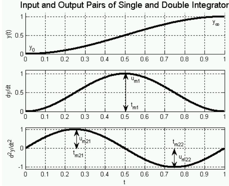
Figure 1.14: MO output  $y$  satisfying (1.18) for  $\varepsilon = \varepsilon_y = 0$  (above) with the corresponding 1P input signal of single integrator  $u_1(t) = \dot{y}(t)$  (middle), or with the corresponding 2P input signal of the double integrator  $u_1(t) = \ddot{y}(t)$  (below)
