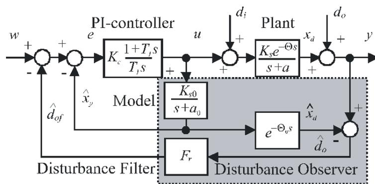
Figure 1.10: Filtered Smith predictor for dead time compensation; Smith (1957) proposed this scheme with  $F_r(s) = 1$
