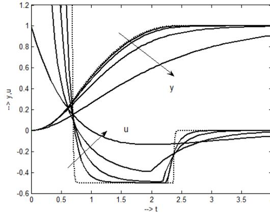
Figure 1.19: Output and control signal transients of double integrator plant by constrained pole assignment control  $U_{max} = 1.2$  and  $U_{min} = -0.5$ ; for double real pole values  $-8, -4, -2, -1$  – arrows indicate pole shifting to zero (i.e. slowing down transients); dotted – MTC transients
