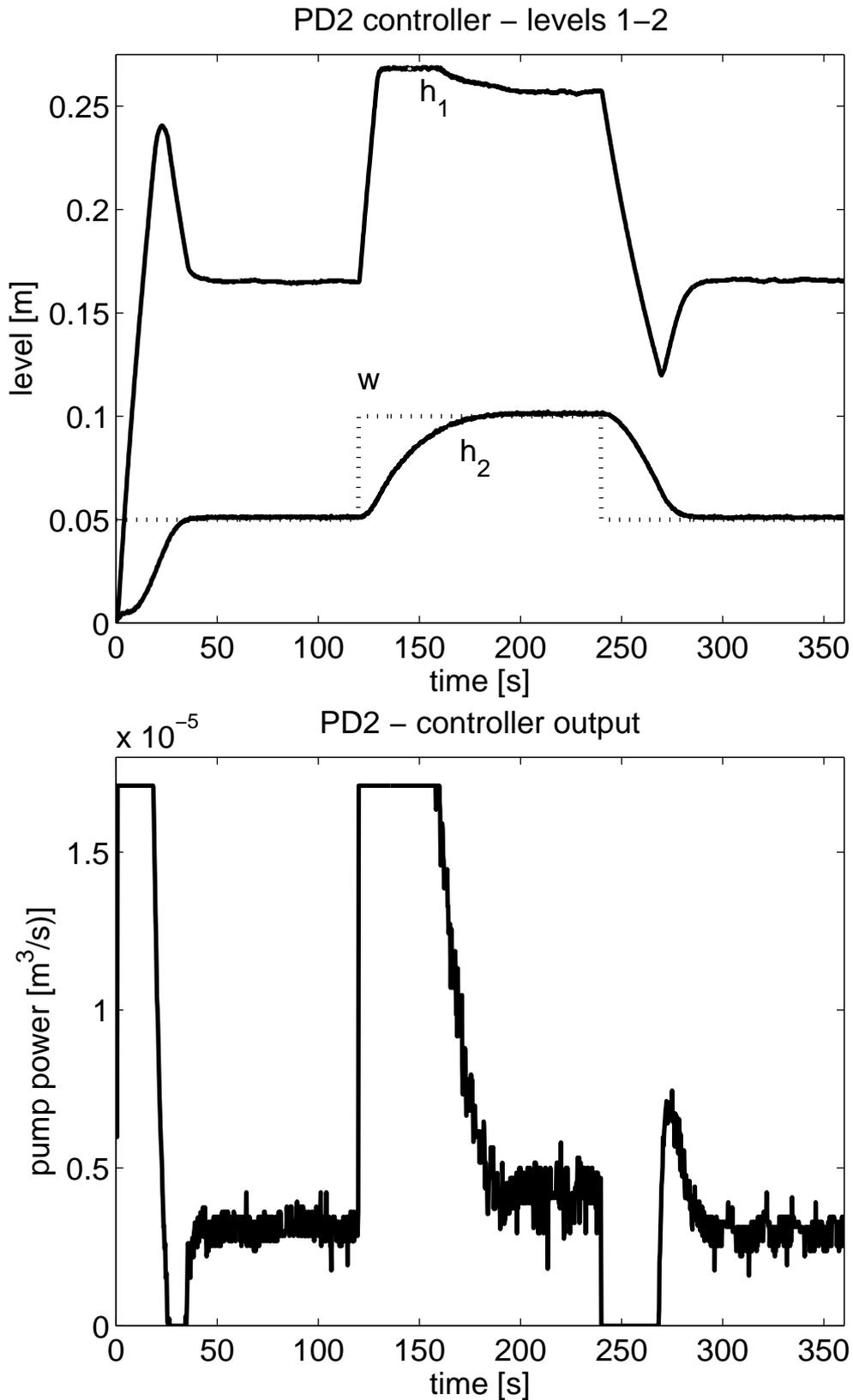
Figure 5.5: Typical setpoint steps in the loop with PD<sub>2</sub> controller with tuning (5.21) may contain up to two step at saturation limits after larger setpoint steps at its output, but for stable systems the 2nd interval at saturation corresponding to braking the transient may disappear or not reach the saturation
