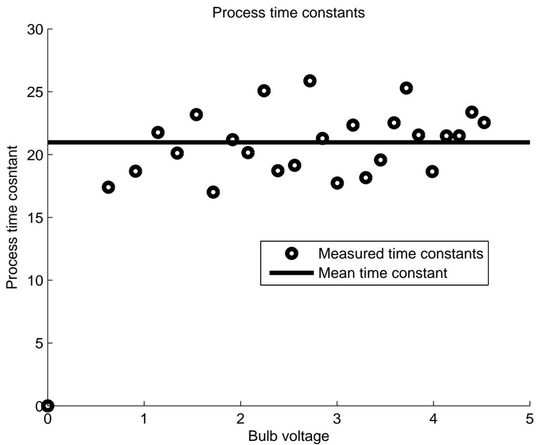
Figure 3.36: Process time constant in several operation points as function of the plant input
