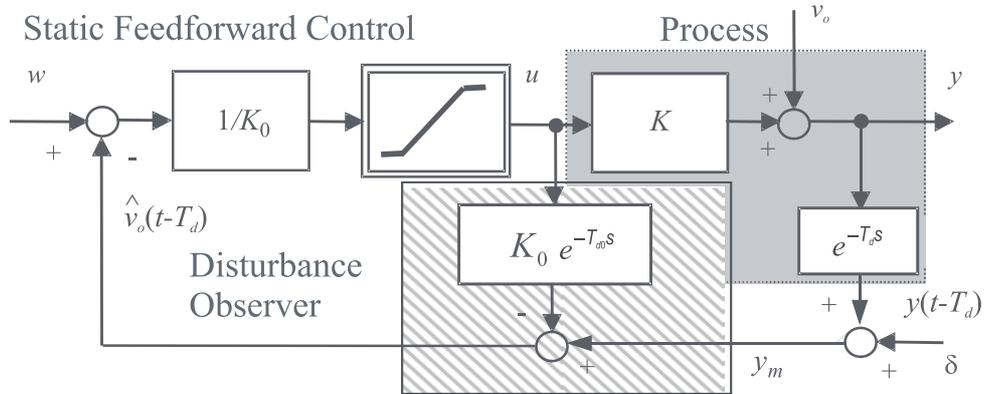
Figure 1.9: Controller for dead time compensation by Reswick (1956)
