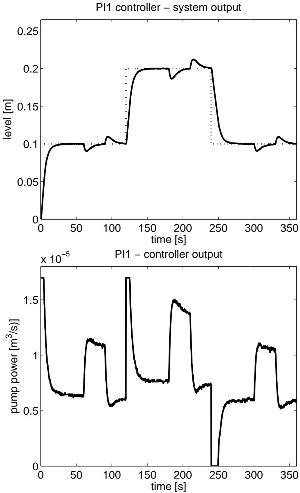
Figure 5.3: Typical setpoint and disturbance steps in the loop with  $PI_1$  controller contain one step at saturation after setpoint steps
