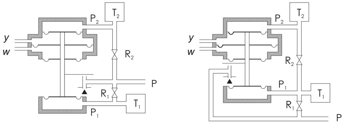
Figure 1.3: Modifications of the pneumatic PID controller with a parallel (left) and a series feedback (right) enabling to achieve different ranges of adjustable parameters and different tuning properties (Ogata, 1997)
