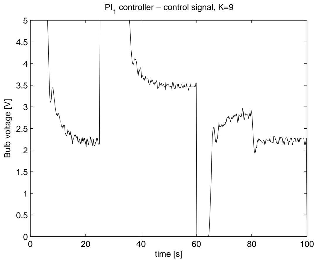
Figure 3.50: PI<sub>1</sub>-controller, filtered light channel control for  $K = 9$
