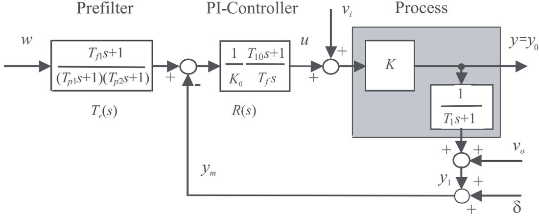
Figure 2.13: Equivalent scheme of the PI<sub>0</sub>-IM controller from Fig. 2.12; tuning  $T_{f1} = T_{p1} = T_f$  gives the 2DOF PI controller with the simplest prefilter  $T_e = 1/(1 + T_{10}s)$
