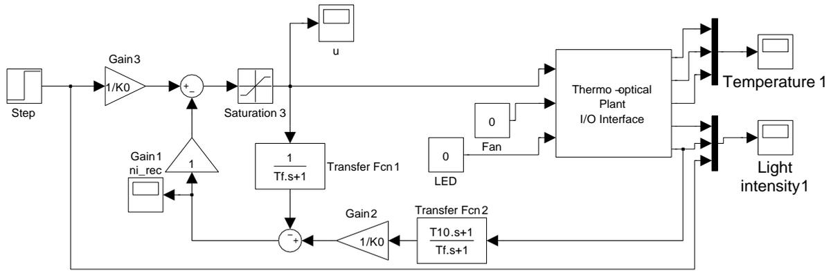
Figure 3.34:  $PI_0$ -controller: Simulink Model; to get  $FPI_0$  controller you need to add pre-filter to the reference setpoint input
