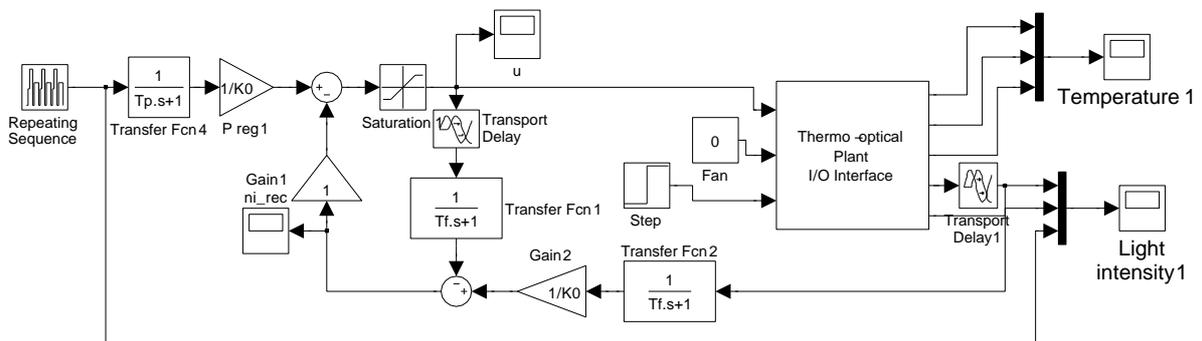
Figure 3.28: FPrI<sub>0</sub>-controller - Simulink model
