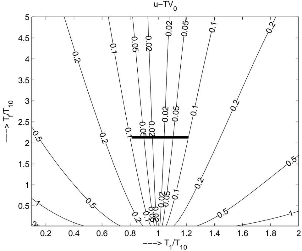
Figure 2.16:  $PI_0$ : Performance portrait for the  $TV_0$  values of the setpoint step responses with the ULS corresponding for the minimal possible value  $\tau_f$  to the limit  $T_1$  values (2.58) and to  $TV_0 < 0.1$
