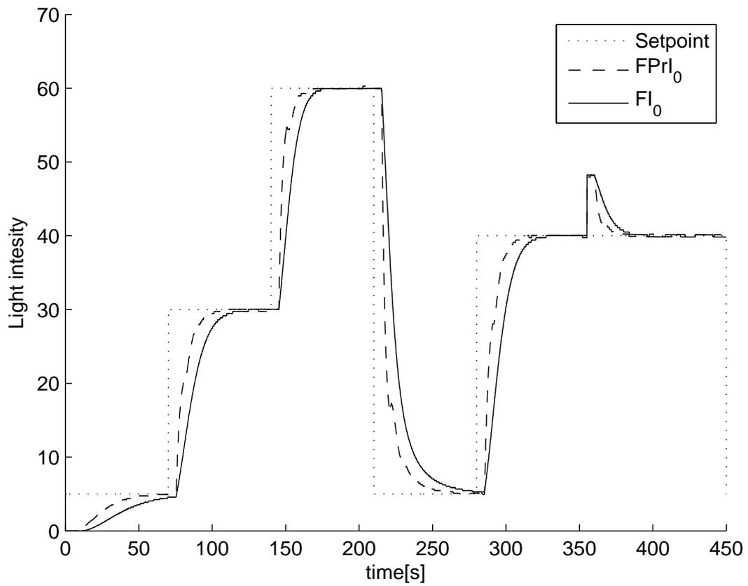
Figure 3.31: FPrI<sub>0</sub> – controller vs FI<sub>0</sub>-controller under 5s transport delay, plant output
