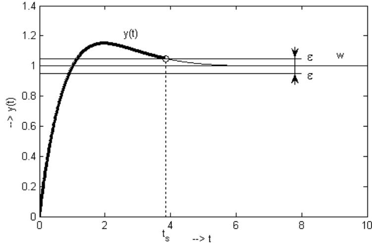
Figure 1.12: Definition of settling time  $t_s$  (1.9) based only on the plant output  $y(t)$  with  $\varepsilon = \varepsilon_y$
