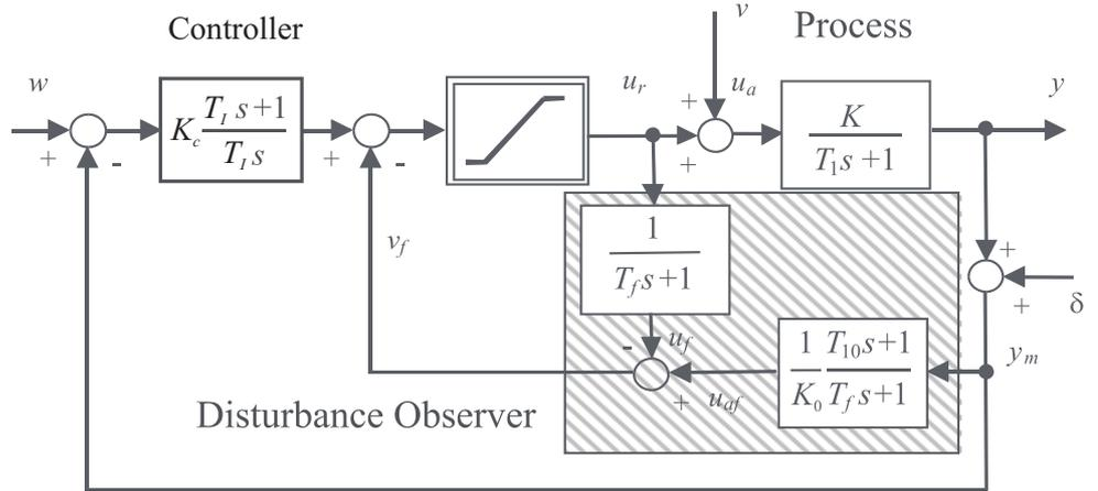
Figure 1.11: Disturbance Observer (DO) based servo-system proposed by (Umeno and Hori, 1991) and interpreted by (Zhao, 2004) as the DO-PI controller
