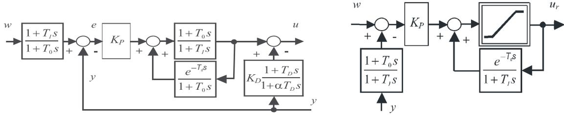
Figure 1.7: Model Driven PID controller (above) (Shigemasa et al, 2002; Yukitomo et al, 2002) that is equivalent to the PPI-PD controller (below)
