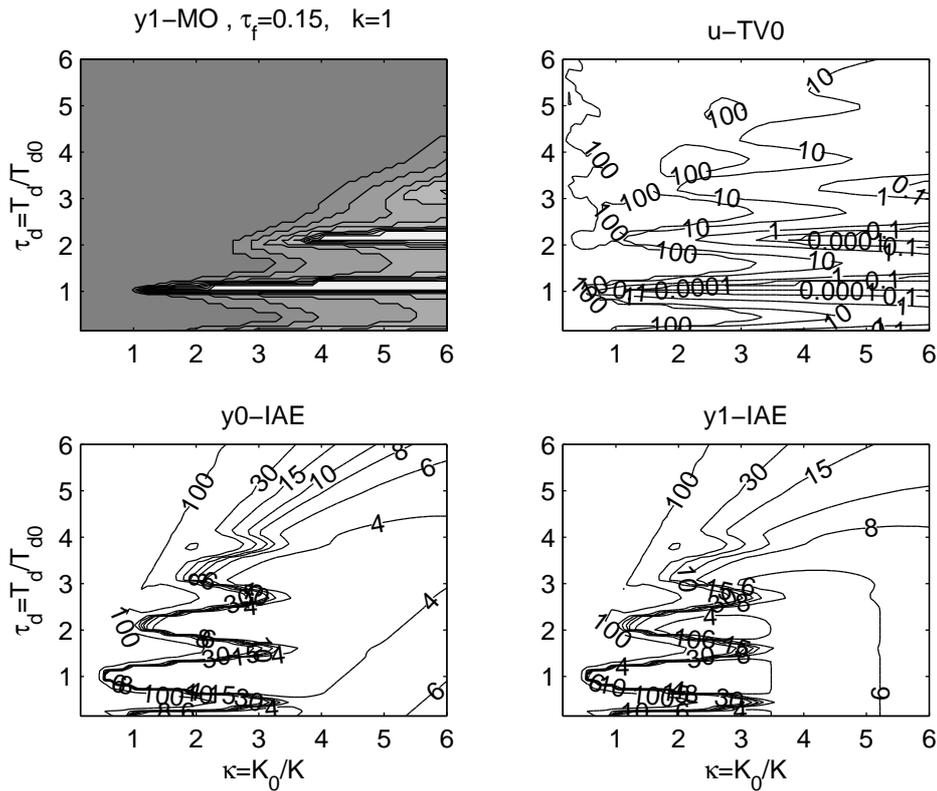
Figure 2.21: Layer of the PP of the plant (2.68) with the FPrI<sub>0</sub> controller corresponding to  $\tau_f = 0.15$  generated over  $61 \times 61 \times 11$  points and showing  $\epsilon_y$ -MO areas (left above) for tollerances  $\epsilon_y = \{0.1, 0.05, 0.02, 0.01, 0.0001, 0.00001\}$ , white denoting the best performance, the  $u$ -TV<sub>0</sub> contours (right above) and the IAE0 and IAE1 levels (below) in the plane  $(\kappa, \tau_d)$
