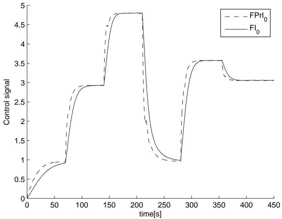
Figure 3.32:  $FPrI_0$ -controller vs  $FI_0$ -controller under 5s transport delay, control signal
