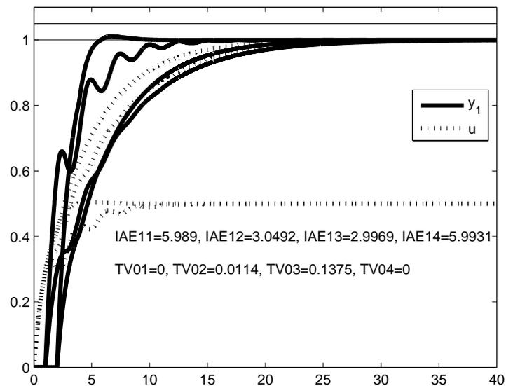
Figure 2.23: Result for seeking an optimal UB of the plant (2.68) with  $K_{min} = 1, K_{max} = 2, T_{d,min} = 1, T_{d,max} = 2$  over PP of 61x61x11 points with identified parameters  $T_f = 1.0648, K_0 = 2.005$  and  $T_{d,0} = 1.8519$ ; areas of  $\epsilon_y$ -MO output step responses identified for tolerances  $\epsilon_y = \{0.1, 0.05, 0.02, 0.01, 0.001, 0.0001, 0.00001\}$ , white denoting the best performance (above) and the corresponding transients (below)
