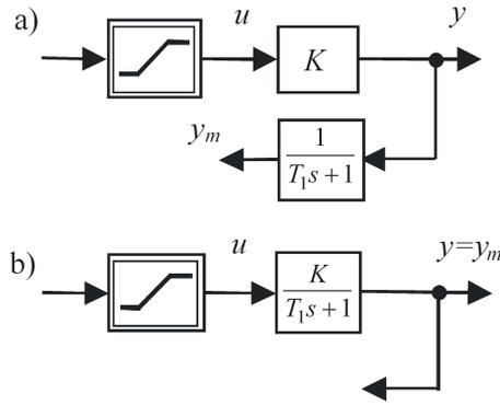
Figure 1.20: Control loops with the 1<sup>st</sup> order dominant dynamics and with relative degrees a) 0 and b) 1.
