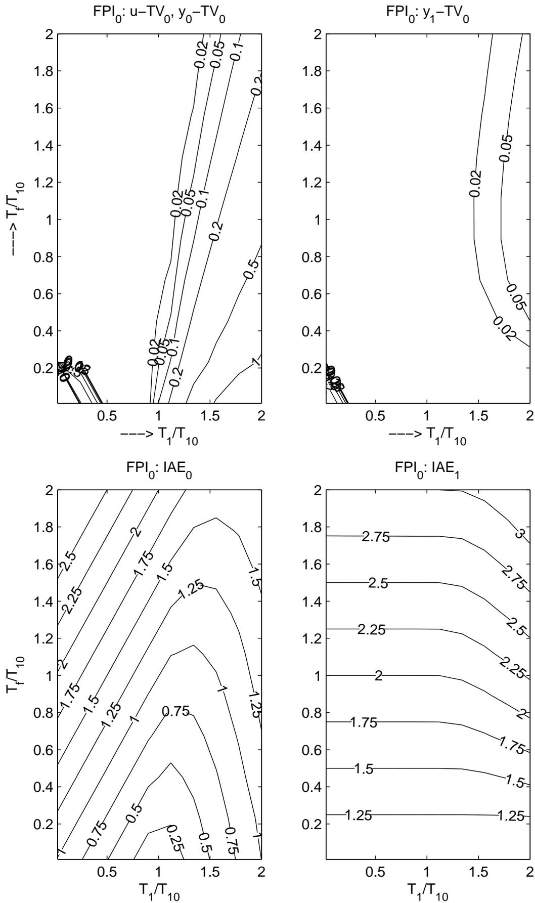
Figure 2.18:  $FPI_0$  with  $T_p = T_f$ : Performance portrait for the  $TV_0$  values of the setpoint step responses at the outputs  $y_0$  (controller output) and  $y_1$  and the equivalent IAE values
