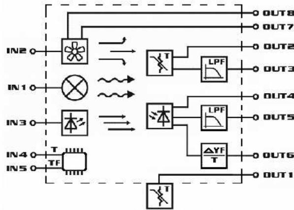
Figure 3.9: Basic electrical diagram of thermo-optical plant uDAQ28/LT
