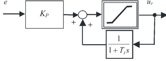
Figure 1.4: Serial implementation of the PI controller considering control signal constraints
