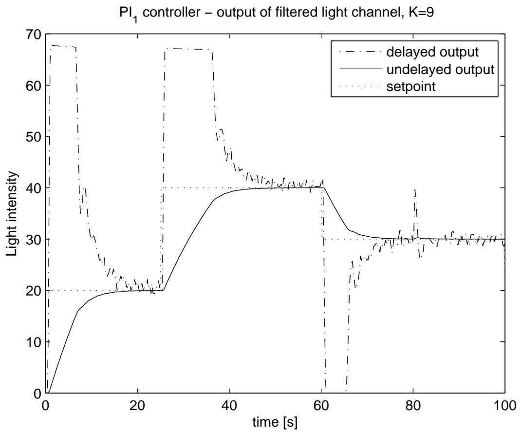
Figure 3.49: PI<sub>1</sub>-controller, filtered light channel control for  $K = 9$
