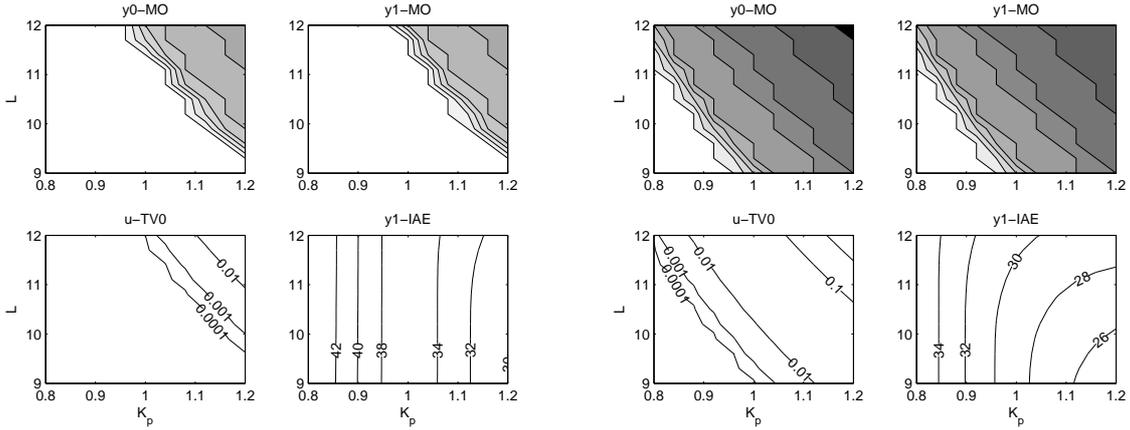
Figure 2.11: PP of the I controller with  $T_f$  tuned to guarantee lower than 2% ( $\epsilon_y = 0.02$ , left) and lower than 10% deviations (right) from MO. MO areas correspond to  $\epsilon_y = \{0.1, 0.05, 0.02, 0.01, 0.001, 0.0001, 0.00001\}$  with white showing the best performance
