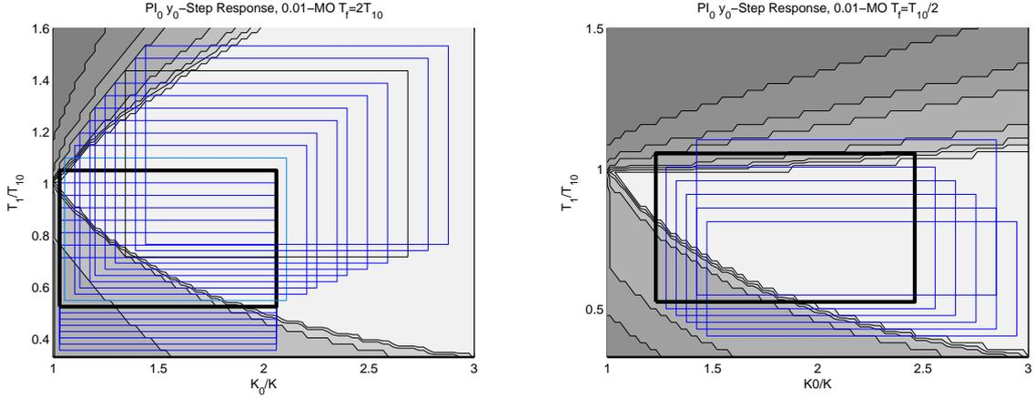
Figure 2.15: Uncertainty boxes corresponding to interval plant parameters (3.43) for  $\tau_f = 2$  (left) and  $\tau_f = 1/2$  (right) and tolerated overshooting 1%; optimal UB (bold)  $\epsilon_y = \{0.1, 0.05, 0.02, 0.01, 0.001, 0.0001, 0.00001\}$  with white showing the best performance;
