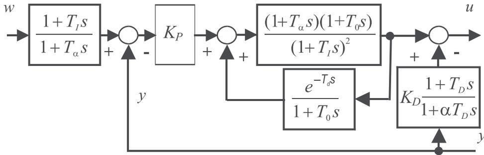
Figure 1.8: 2DOF MD-PID controller
