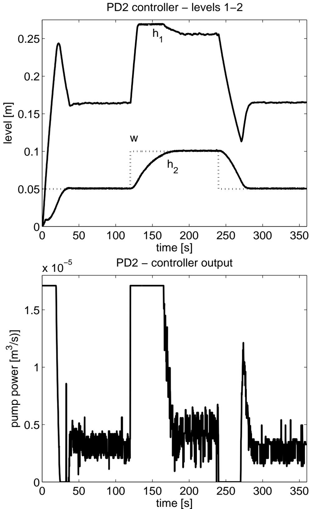
Figure 5.6: Typical setpoint steps in the loop with PD<sub>2</sub> controller with tuning (5.22) derived by the performance portrait method Huba (2011b) gives a bit tighter control and faster dynamics of transient responses than the traditionally used tuning (5.21) what may be e.g. observed by longer period at the maximal level of  $h_1$  in the first tank and yet more by higher noise amplification
