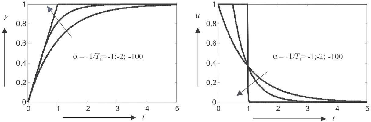
Figure 5.1: Impact of the P controller tuning on the transient responses
