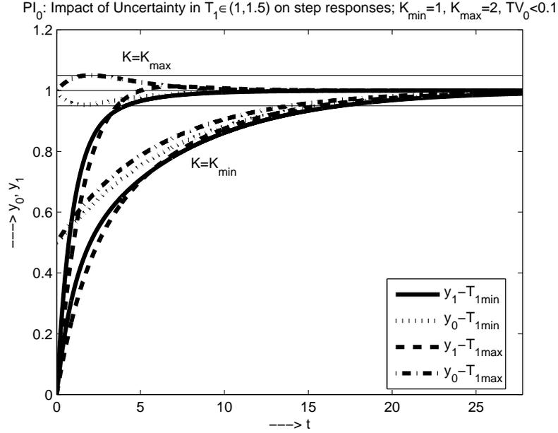
Figure 2.17: PI<sub>0</sub>: Setpoint step responses corresponding to limit values (2.58) and satisfying  $TV_0 < 0.1$  show amplitude deviations from monotonicity  $\epsilon_y \approx TV_{0,max}/2$
