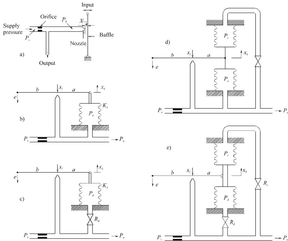
Figure 1.1: Modular concept of pneumatic PID Control. a) Flapper-Nozzle high gain nonlinear amplifier, b) P controller, c) PD controller, d) PI controller and e) PID controller (see e.g. Ogata (1997); Van de Vegte (1994))
