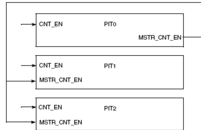
Figure 16-3. CNT\_EN Connection Between Multiple PITs
