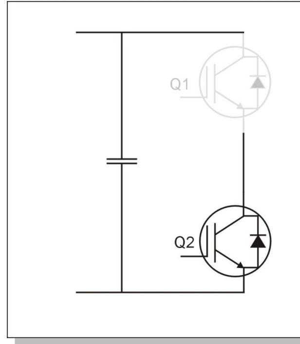
The top or bottom transistor is switched during whole period.
