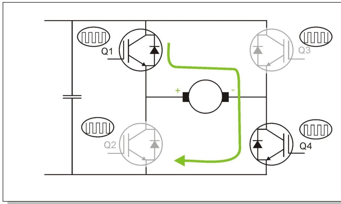
$Q1 = 50\% \pm DC$ ;  $Q4 = 50\% \mp DC$ ;  $Q2 = \overline{Q1}$ ;  $Q3 = \overline{Q4}$ ;  $DC$  – *duty cycle*
