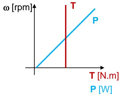
Mechanical characteristics of a crane
