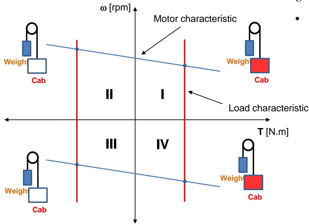
$$Weight = Elevator\_cage + \frac{1}{2} Load$$
