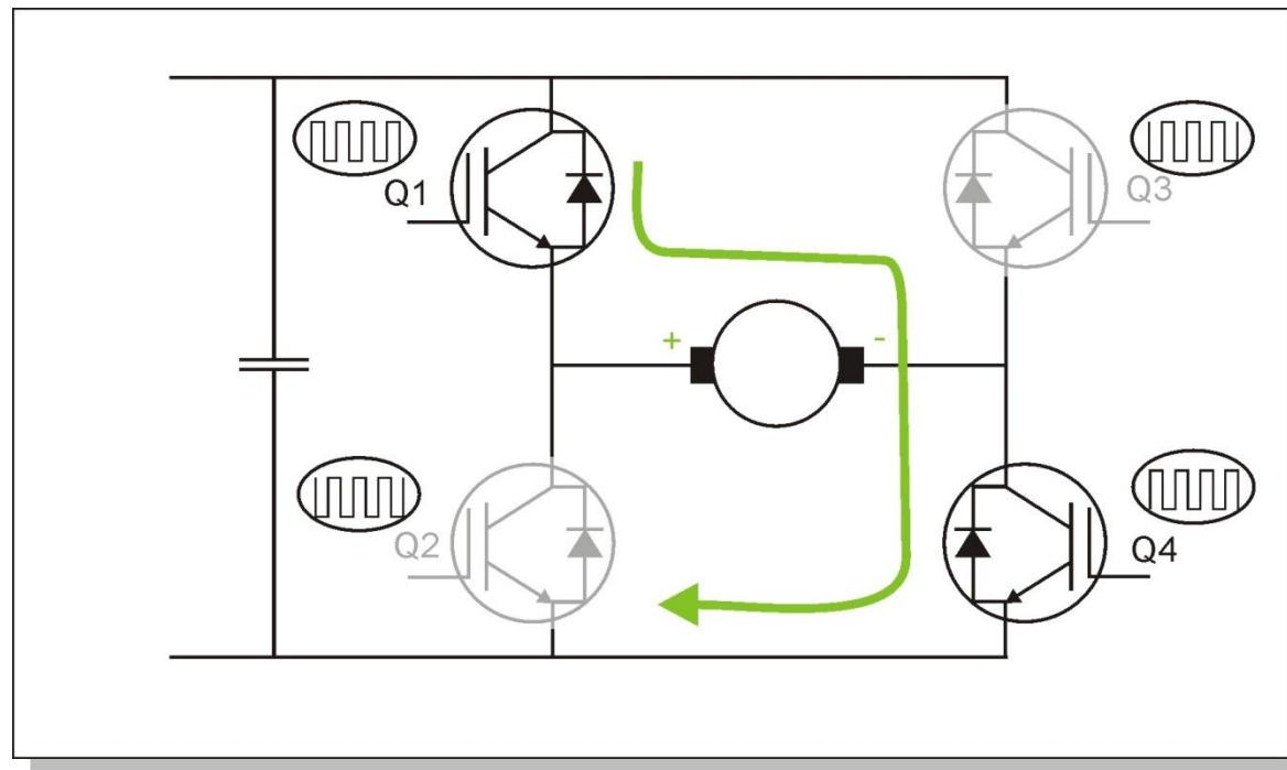
$$Q1 = Q4 = \text{PWM}; Q2 = Q3 = \overline{Q1}$$
