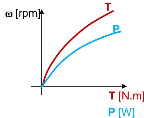
Mechanical characteristics of a fan
