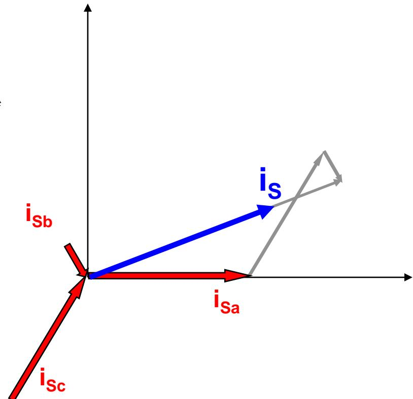
We are able to generate stator field to any position over 360°
