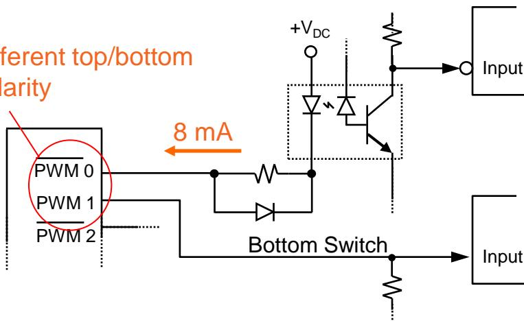
Direct PWM pin-optocoupler connection
