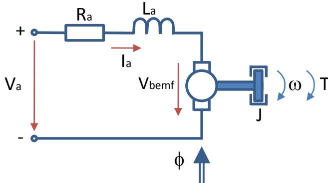
**Equation describing dynamics of electric circuit**
