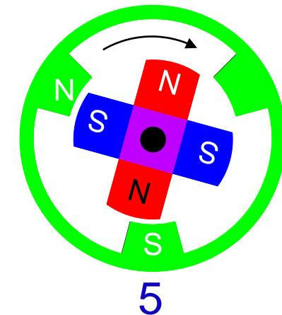
One phase is unpowered at any given time.
