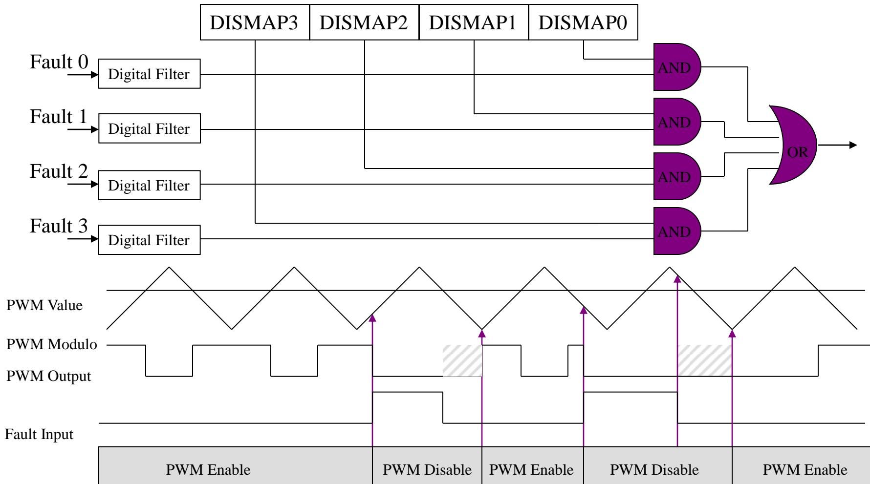
\*When Fault logic returns to logic 0, the PWM restart at beginning of the next half cycle.
